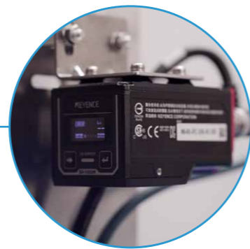
The 2D code reader scans the code on the pcb and enables the automatic loading of the correct printing program
