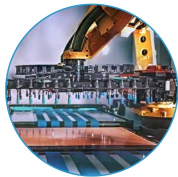
Fully automated inkjet solder mask system cluster
